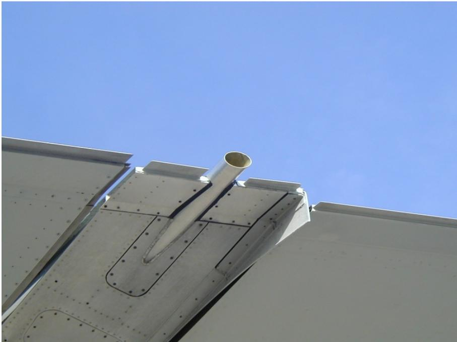
Figure 2 Fuel dumping nozzle of an Airbus A-330
